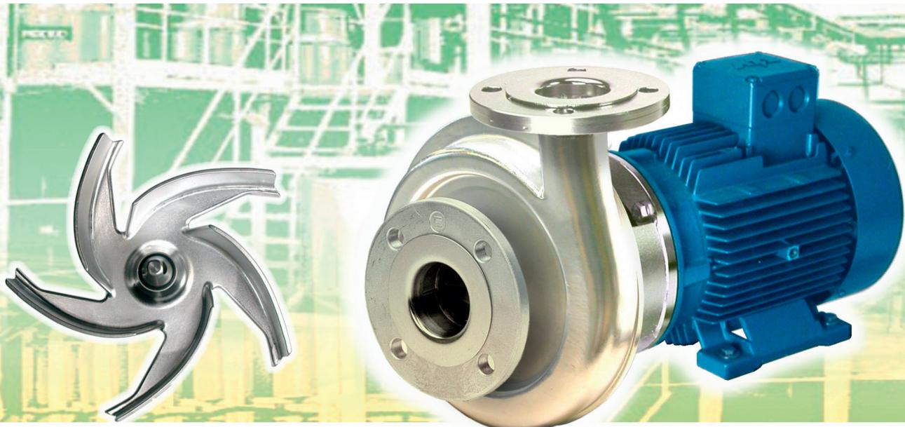
The **MWP2-40** series provide a robust wear resistant pump construction. The pump casing is made of thick-walled cast duplex stainless steel. This means that the **MWP2** is particularly suitable for the transfer of abrasive liquids. Typical applications are the circulation of liquid feeding for animals and diatomaceous earth (Kieselgur) for filtration purposes, where the **MWP2** range has proven its reliability for more than 25 years.
