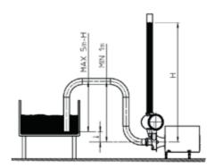
Since an air-handling pump has no water retaining vessel, special attention has to be paid to the pipe work in case the pump is not
