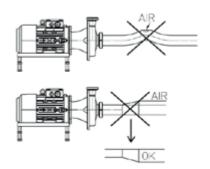
To prevent air traps, the suction pipe must contain no bridges (a part of a pipe that has both ends lower than the middle) and should have an ascending gradient of 1 % toward the pump. Pipe reducers should be of an eccentric type and installed so that no air can be trapped (not for MSP, SCP, ISP, CRP, PRP and IRP). Install the suction pipe in a way that the liquid flows automatically into the pump. (Not for self-priming pumps MSP, SCP and ISP)
