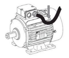
Connect according to the coupling information on the identification plate and the diagram in the terminal box. Do not connect
