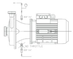
For **type P** (double pressurized seal) quench configuration the pressure in the quench chamber must always be at least 1 bar higher than the pressure on the inlet of the pump for pumps with open impeller and at least 4 bar higher than the pressure on the inlet of the pump for pumps with semi-open or closed impeller.
