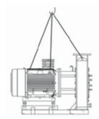
When the sling has been removed, the pump may only be lifted on the eyebolt of the motor. If the pump casing is provided with a lifting Put down the pump carefully in order not to damage the internal parts.
